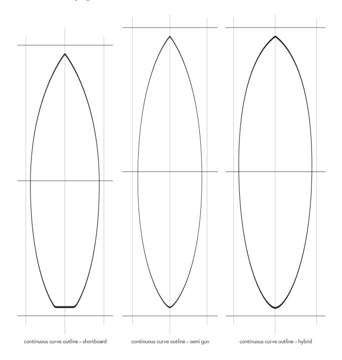
"Hybrid" outlines feature combinations of strong paralle lines and smooth continuous curves in the distribution and configuration of the surface area of the surfboard. They are common to all classes of surfboards. (Shortboards, semi guns, big wave guns, tow boards, hybrids, funboards, and longboards.)
