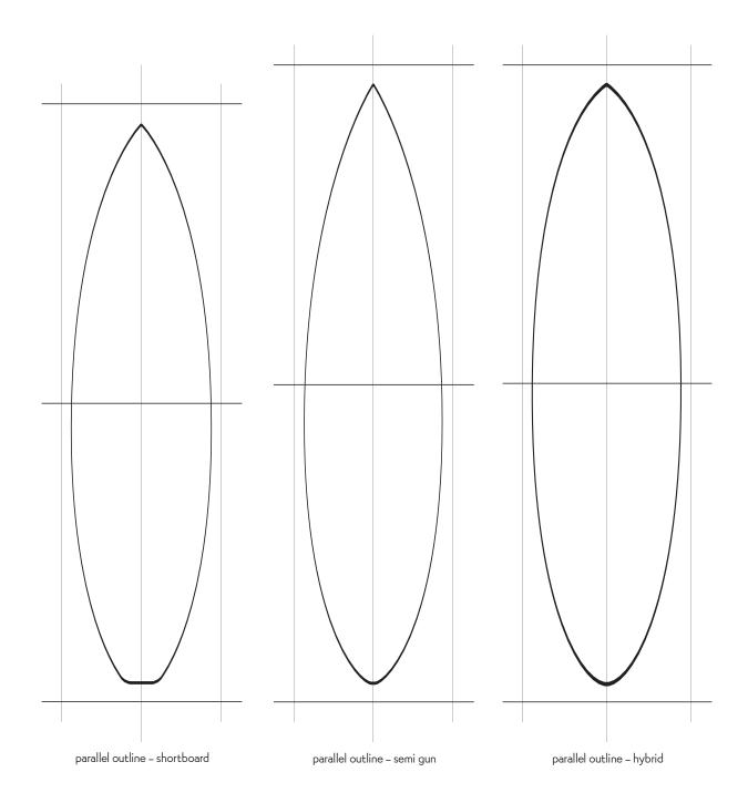
Illustrations of three parallel outlines, applied to shortboards, semiguns, and hybrids. Note the strong – nearly straight – curves carrying from the widepoint towards the nose and tail in each of the designs.
